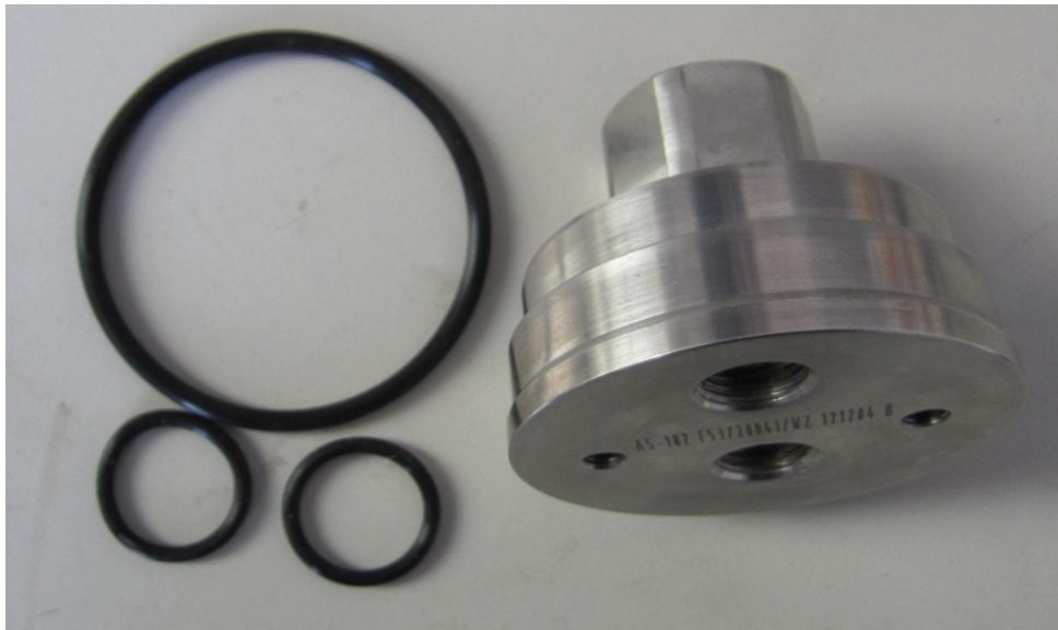
Figure 2.7 Head breakdown Components: End Cap and seals.
