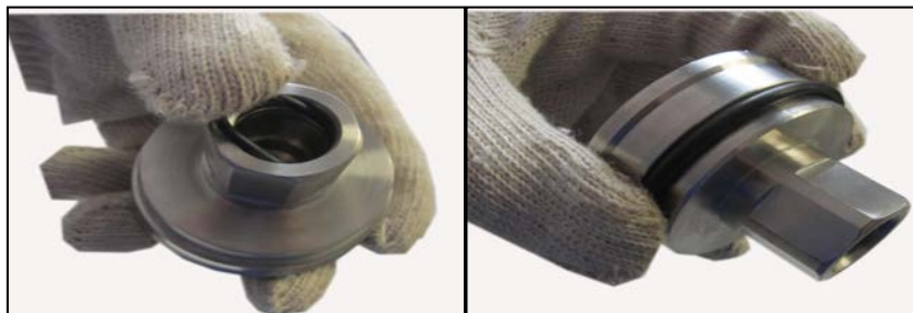
Figure 2.8 Install the permeate and end cap seal.
