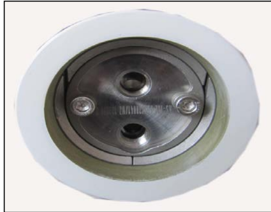
Figure 2.11 Install retaining ring and screws
