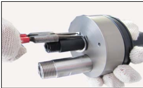
Figure 2.7 Remove retaining ring
