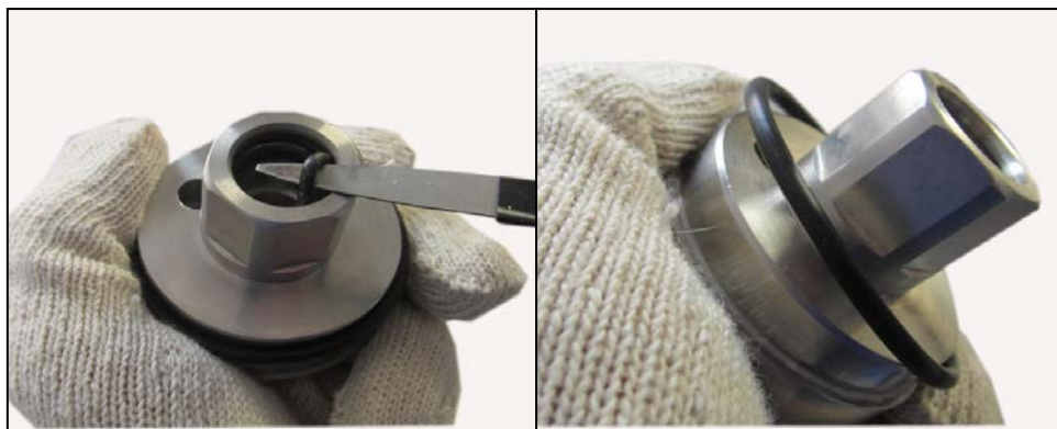
Figure 2.6 Remove adaptor and seals
