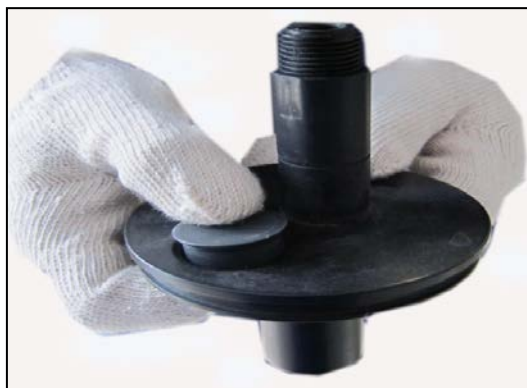
Figure 2.12 Install the seal plate plug.
