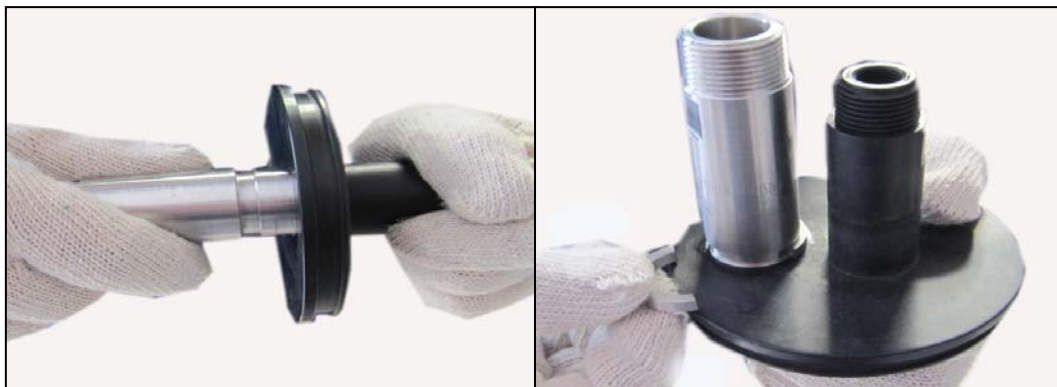
Figure 2.13 Feed/concentrate port installation.
